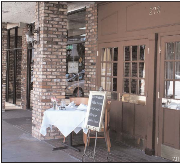
WIDE SIDEWALKS: Enough sidewalk depth is especially important for restaurants to create a pleasant environment for would-be customers. Street dining requires enough separation from the street to allow for pedestrians to pass by tables. Good depths for sidewalks in urban conditions are a minimum of 12 feet.
