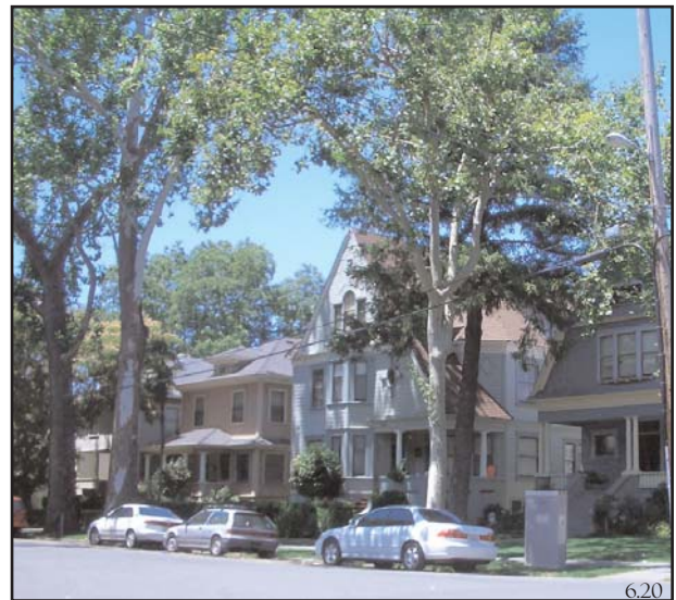
RESIDENTIAL STREET, CHICO, CA: Residential streets with minimal commercial activity have different requirements than their urban counterparts. 6-8 foot planting strips with tall street trees are encouraged. Houses are detached with porches in front facing the street. Parking is placed on street and in alley-loaded garages.
