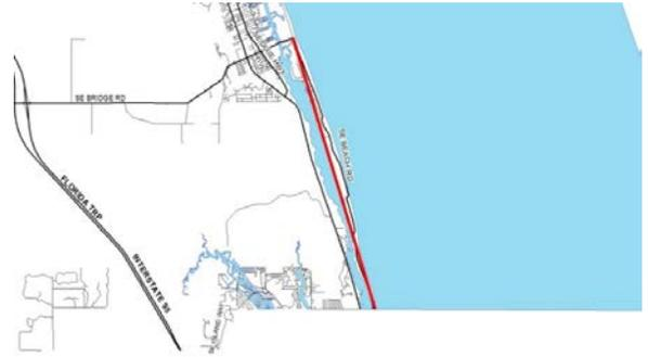
**Project Limits** Milling, resurfacing, widening of 7.1 miles of South Beach Road.
