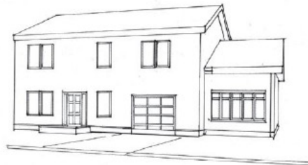
A garage door no wider than 30 percent of the width of the front wall plane will maintain an acceptable scale along the street front.
