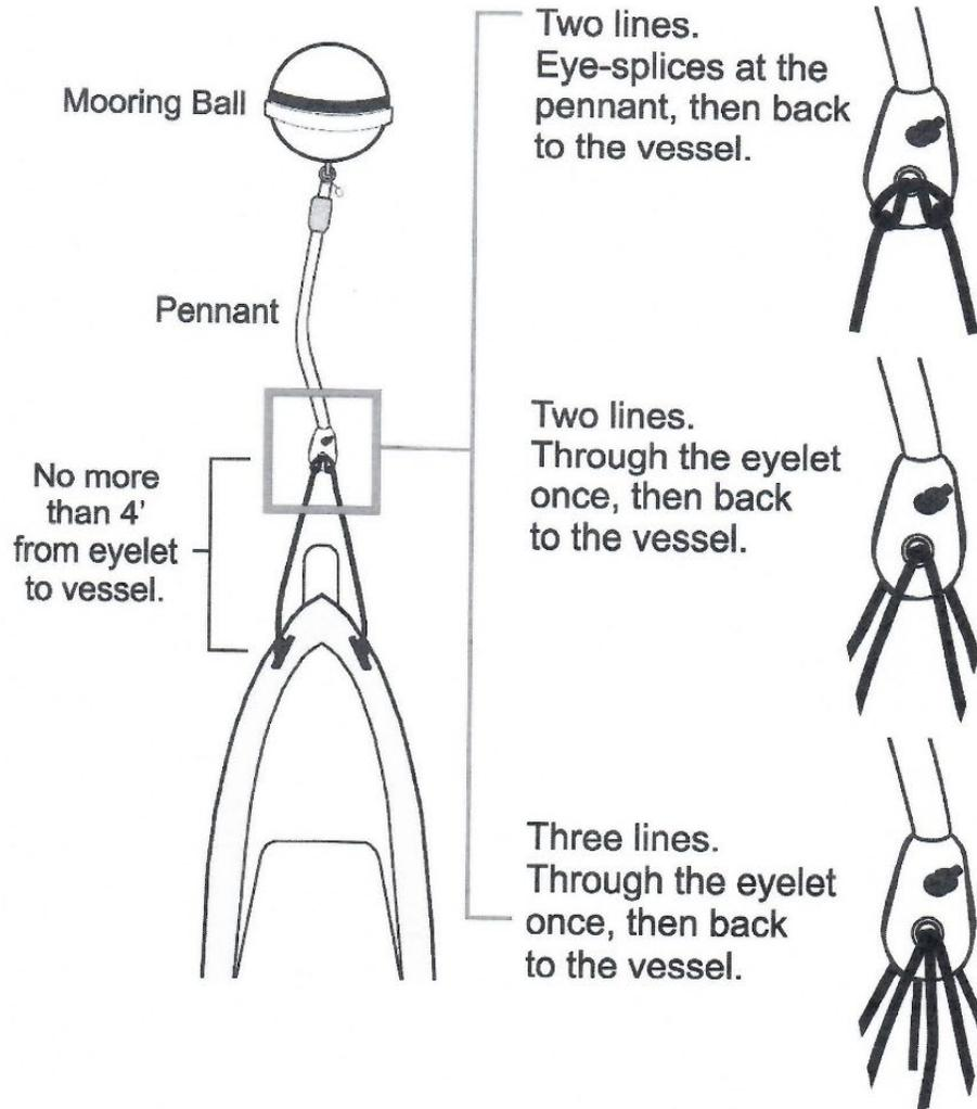
**EYELET AND FLOAT MUST STAY OUT OF WATER**
